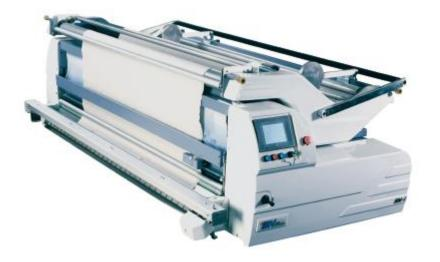
Tension free spreading with auto feeding cradle, lay the knitting and woven fabric down in a perfectly aligned edges.
